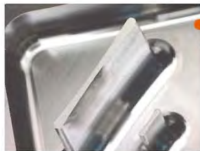
R1×8加工后刀具图片 Cutting edge after machining
