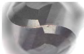
刀具磨损量 0.014mm Tool wear
