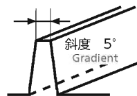
R1×4加工后刀具图片 Cutting edge after machining
